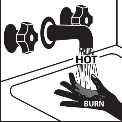
Water temperature over 125°F can cause severe burns instantly or death from scalds. Children, disabled and elderly are at highest risk of being scalded. See instruction manual before setting temperature at water heater. Feel water before bathing or showering. Temperature limiting valves are available, see manual.
