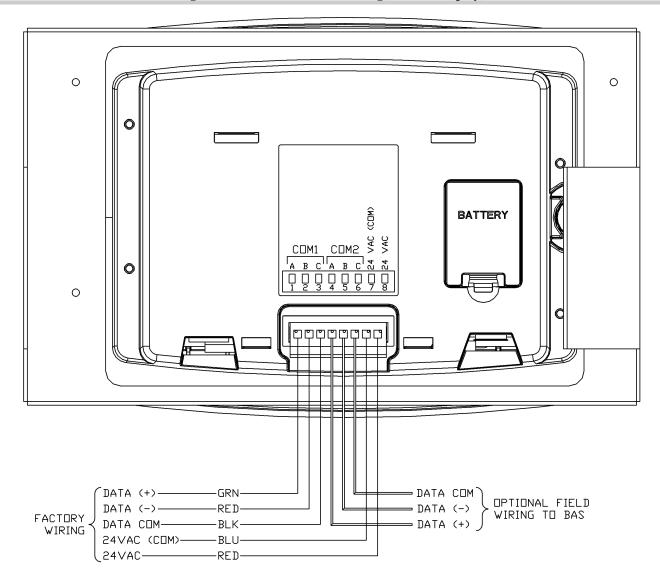
Figure 12-3 COM2 Modbus Wiring (Rear of Display)
